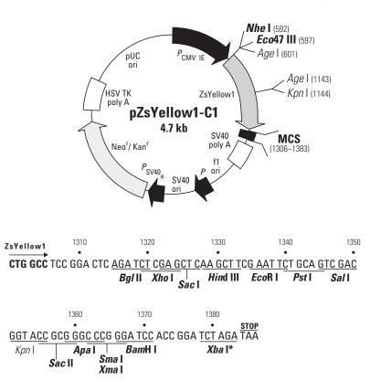
**Restriction Map and Multiple Cloning Site (MCS) of pZsYellow1-C1.** Unique restriction sites are in bold. The *Xba* I site (\*) is methylated in the DNA provided by CLONTECH. If you wish to digest the vector with these enzymes, you will need to transform the vector into a *dam*<sup>-</sup> host and make fresh DNA.
